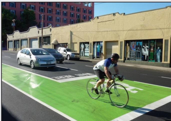
Bike Boxes are a new kind of street marking to help motorists and cyclists share the road. Bike boxes are used at intersections to designate a space for cyclists to wait in front of cars at a red light and then proceed first through the intersection when the light turns green. Once they clear the intersection they resume travelling in the bike lane.
