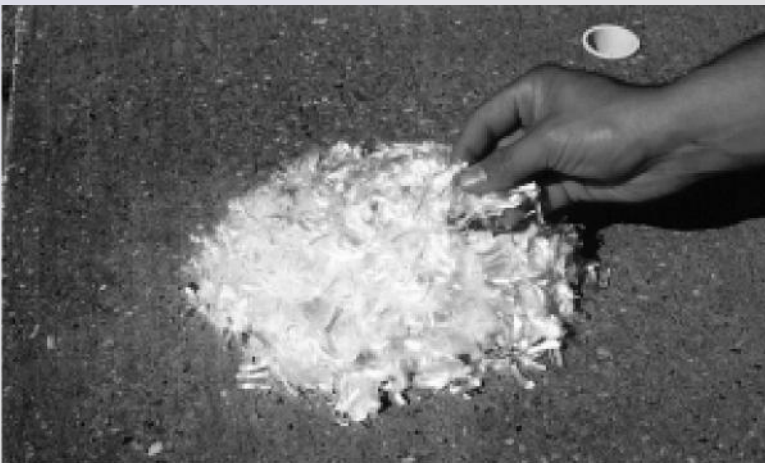
Figure 1-13: Synthetic fibres are added to concrete mixtures at a rate of about 0.3 to 1.2 kg per cubic metre.
