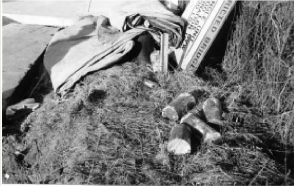
Figure 1-36: Improper storage of cylinders (as shown here) will make test results invalid.
