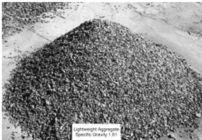
Figure 1-6: These lightweight aggregates were used in concrete that had a unit weight of 1800 kg/m 3
