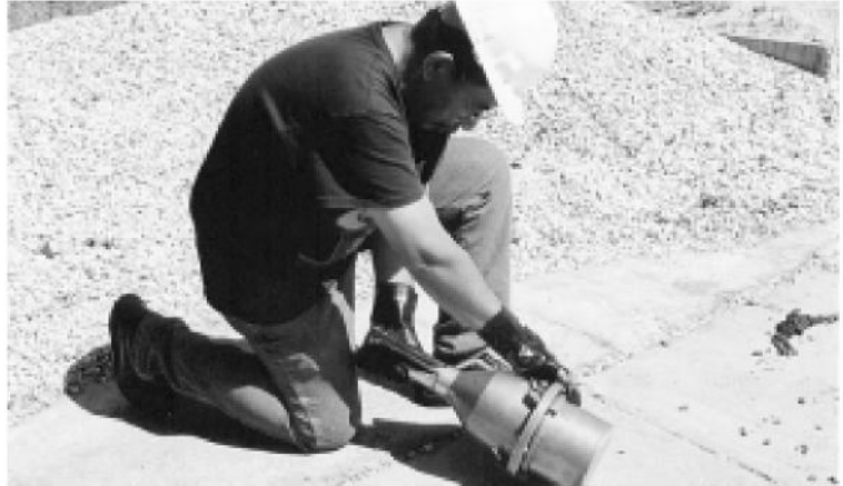
Figure 1-32: The volumetric air meter does take significant effort to obtain an accurate air content measurement.
