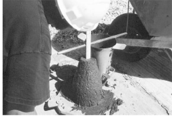
Figure 1-29: The slump of the concrete should be measured to the nearest 5 mm.
