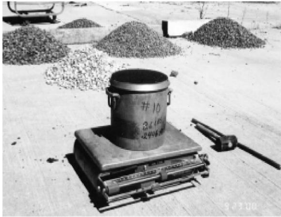
Figure 1-27: Concrete is sold by volume. Concrete yield is calculated from the density.
