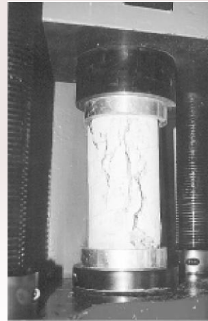
Figure 1-34: Generally, concrete test cylinders are broken in the lab after 28 days to ensure that concrete meets the job requirements, or for quality control.
