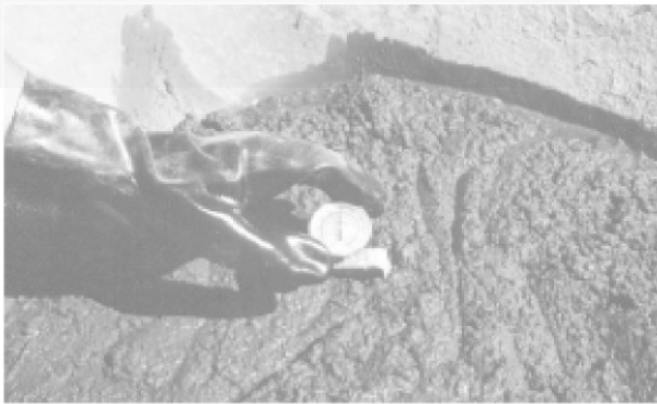
Figure 1-26: The thermometer must be inserted into the concrete at least 75 mm when the temperature is measured.
