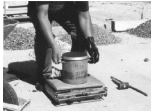
Figure 3-6: The density test is the primary test that should be used to solve yield problems.
