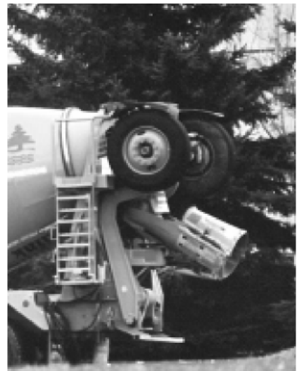
Figure 4-17: If the truck is stuck and is in danger of tipping over, a CDP may consider using the booster axle to help stabilize the
