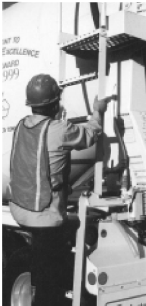
Figure 4-8: Always maintain at least three points of contact when climbing truck ladders.
