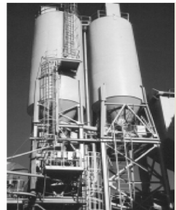
Figure 4-11: Cement silos and aggregate bins are considered confined spaces.
