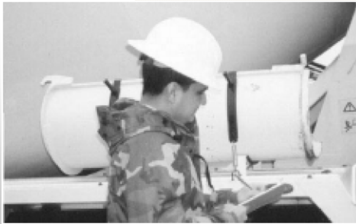
Figure 4-13: Extension chutes should be strapped while not in use, which prevents them from falling off the truck mixer.
