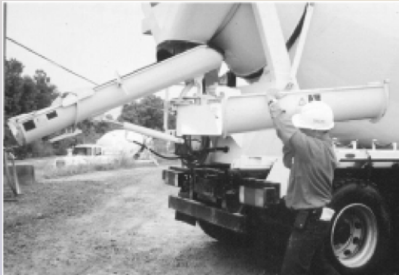
Figure 4-2: Proper lifting technique should always be used when placing extension chutes on the mixer.
