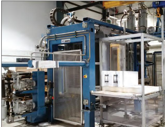
Newfoundland Styro uses this Kurtz ICF machine to manufacture its insulated concrete forms
