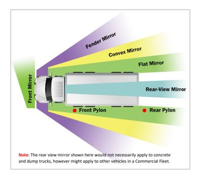
Start by placing one pylon approximately 10' behind the flat mirror on the driver's side and space it approximately 12" from the side of the vehicle. Then place the second pylon in-line with the first pylon approximately 10' behind the vehicle. Repeat this process on the passenger side.
