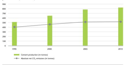
Perimeter of  $CO_2$  emissions considered: only direct  $CO_2$  emissions related to the production of cement and clinker, excluding on-site electricity production.
