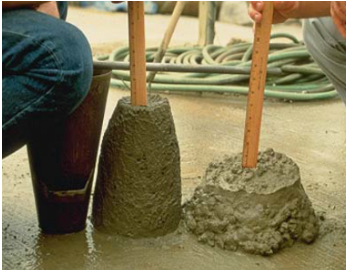
Concrete with varying slumps
